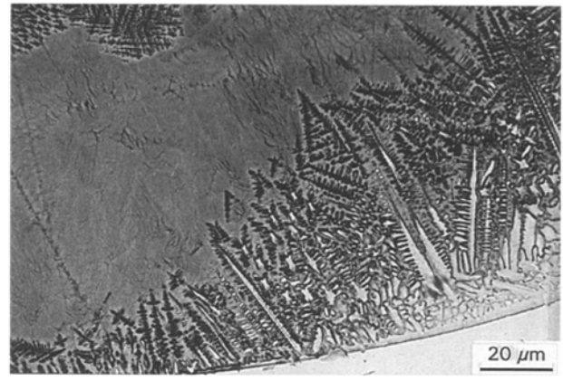
Figure 5 Secondary electron image of sample 2b (316L-C) showing the dendritic and eutectic structures (s.c. = 5 \text{ mg cm}^{-2} , P = 200 \text{ W} , v = 5 \text{ mm s}^{-1} ).
