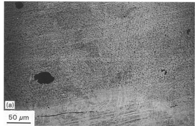
Figure 4 Sample 2a (316L-C): s.c. = 2 \text{ mg cm}^{-2} , P = 200 \text{ W} , v = 5 \text{ mm s}^{-1} . (a) Secondary electron image showing the dendritic microstructure. (b) Secondary electron image showing the eutectic in the interdendritic areas.
